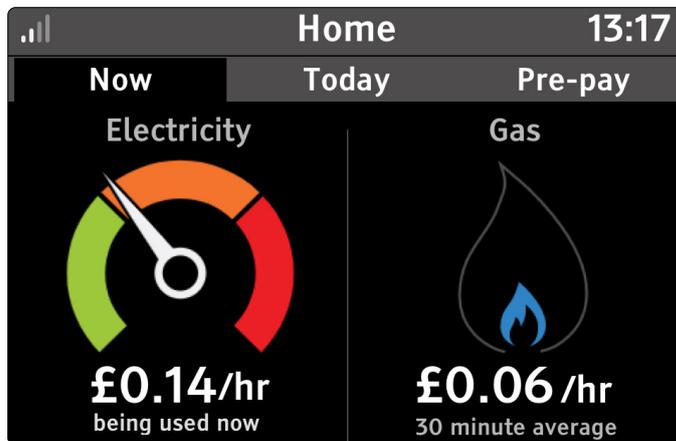
The dial on the left (only available when you have an electricity smart meter) shows the current rate of electricity energy use for your home.
