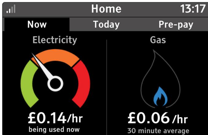
The **Now** screen is split into two parts and indicates the consumption now. **Electricity** is displayed on the left and **Gas** on the right.
