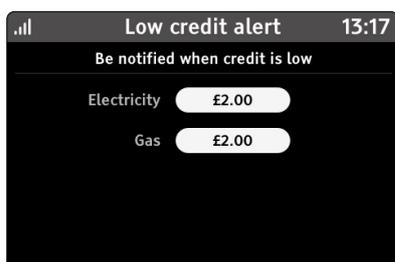
If set by the meter it is not possible to set the alert lower than the meter value. The amount can be changed for each fuel by selecting the appropriate fuel and entering a value. Only fuels in prepayment mode are shown.
