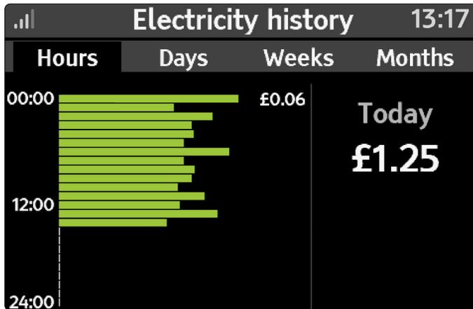
The **Electricity usage history** has four tabs, from left to right: Hours, Days, Weeks and Months. Use the left and right arrow keys to move between the tabs.
