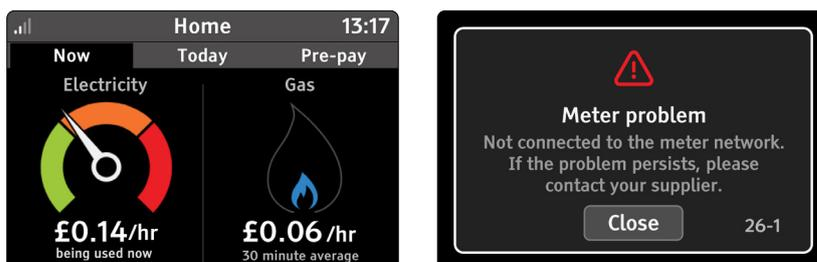
If your Smart Display loses connection to the smart meter(s), then it will show the alert above. Try moving the Smart Display closer to the electricity smart meter to reconnect.
